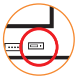
2-1 Clear CMOS Jumper CLR-CMOS
