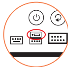
2-1 Clear CMOS Jumper CLR-CMOS
