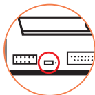
2-1 Clear CMOS Jumper CLR-CMOS
