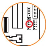
2-1 Clear CMOS Jumper CLR-CMOS
