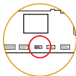
2-1 Clear CMOS Jumper CLR-CMOS
